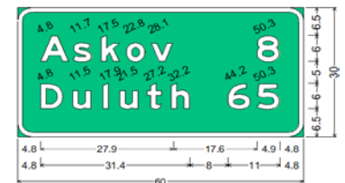
Askov 8 Duluth 65; 3.0" Radius, 1.0" Border, White on, Green; "Askov", E Mod 2K; "8", E Mod 2K; "Duluth", E Mod 2K; "65", E Mod 2K;
