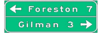
L1 ARROW FORESTON 7 GILMAN 3 RT ARROW: 6.0" Radius, 1.0" Border, White on, Green; Arrow L, 13.0" H80; "Foreston 7", E Mod 2K; "Gilman 3", E Mod 2K; Arrow R, 13.0" W;
