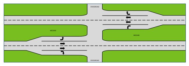
Figure 1.1 - Standard At-Grade Expressway Intersection Layout
