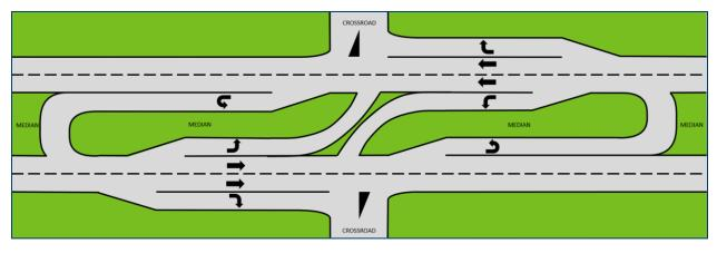
Figure 1.2 - Standard At-Grade Expressway Intersection Layout
