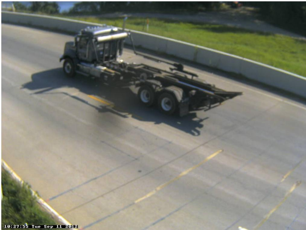
Photo 10B: Class 6, 3 axle, Single Unit; Dumpster Hauler, No Dumpster.
