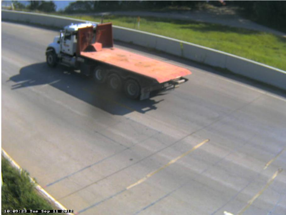
Photo 12A: Class 6, 3 axles, Single Unit; Flatbed, Empty.
