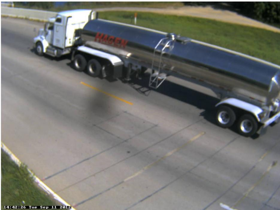
Photo 33B: Class 9, 5 axle, Semi-Tractor with Trailer; Tanker; Food; Dairy.
