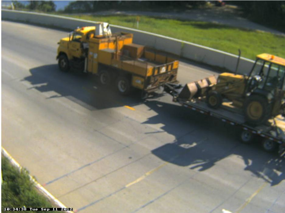
Photo 29A: Class 9, 5 axle, Truck with Trailer; Service Truck; Construction; Utility: w/Construction Equipment.
