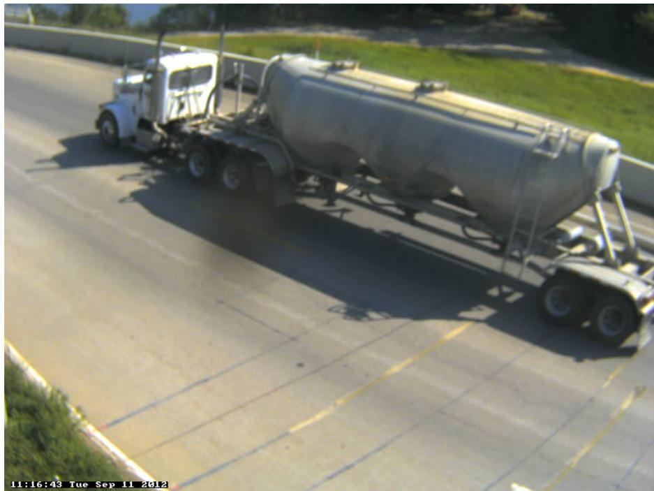
Photo 31B: Class 9, 5 axle, Semi-Tractor with Trailer; Tanker; Dry Bulk Tanker.
