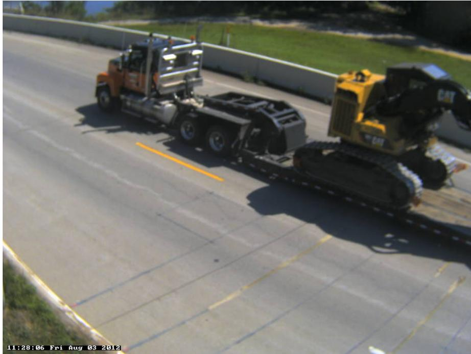
Photo 24A: Class 9, 5 axle, Semi-Tractor with Trailer; Low Boy; Construction Equipment.
