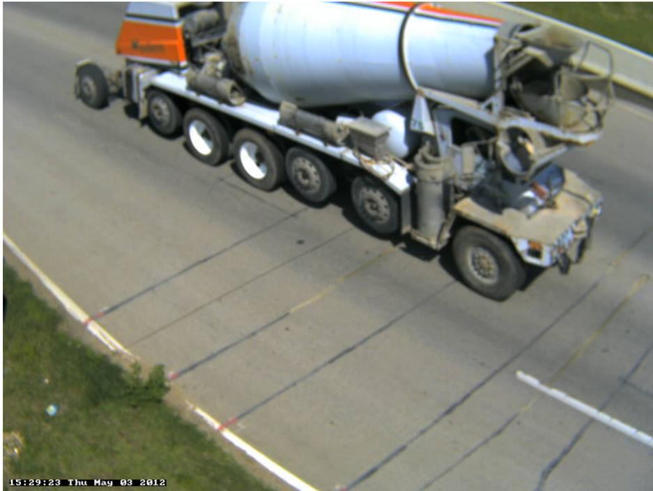
Photo 7B: Class 7, 4+ axle, Single Unit; Construction; Concrete Truck.
