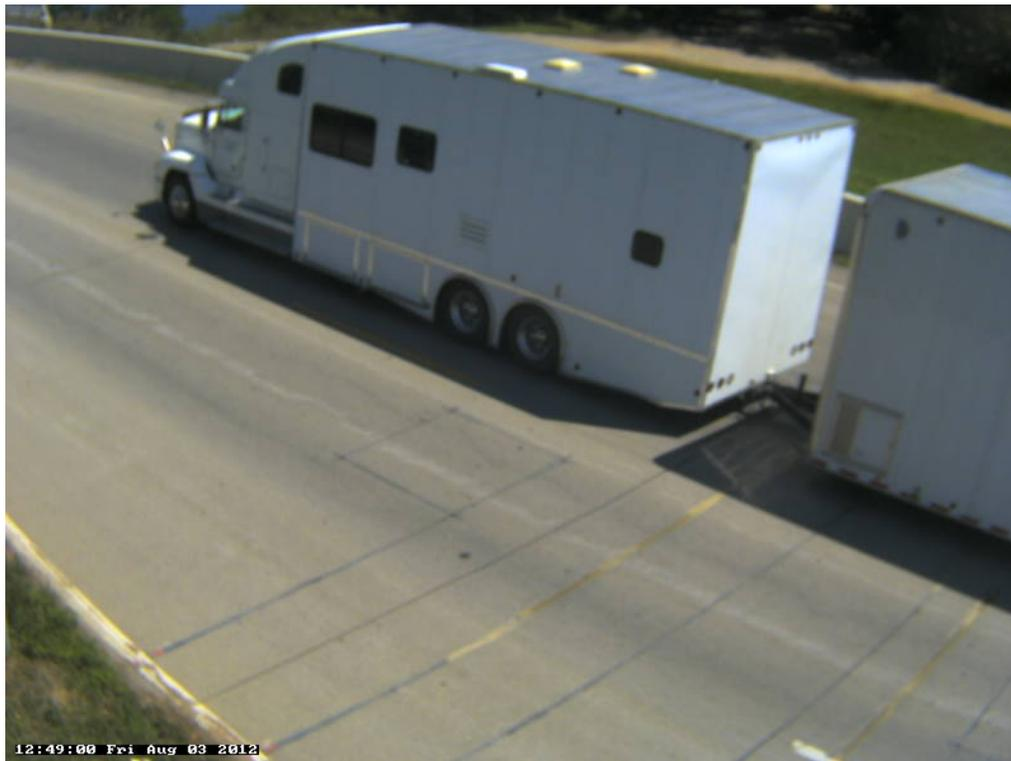
Photo 4B: Class 6, 3 axle Truck and Trailer; Box.
