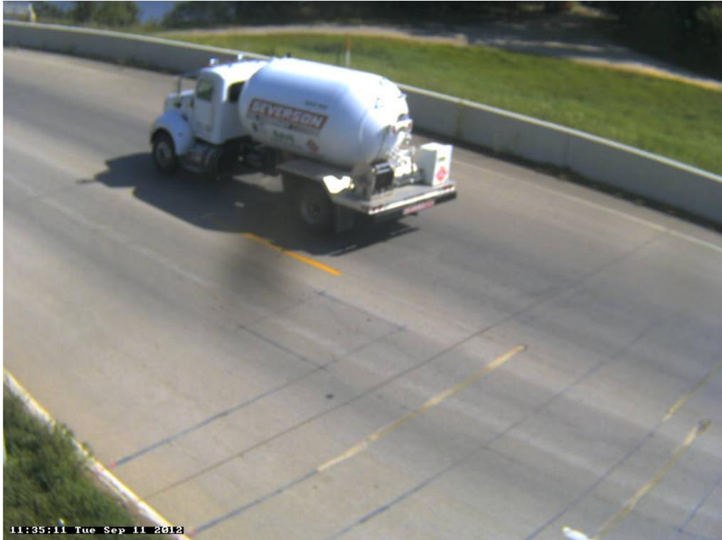
Photo 35A: Class 5, 2 axle, 6-tires, Single Unit; Tanker; Fuel; Propane or Liquid Natural Gas (LNG).
