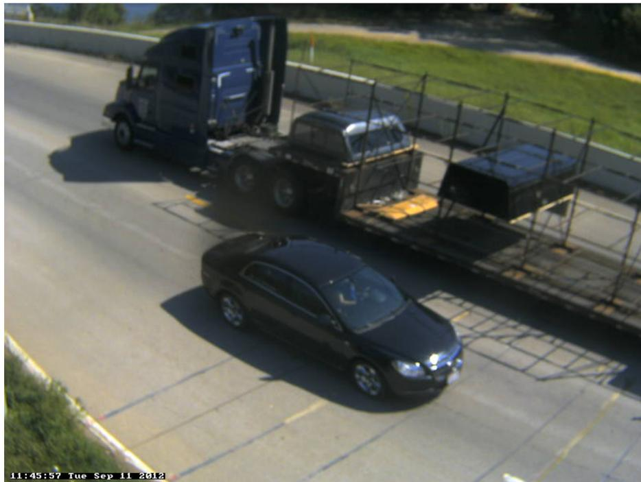
Photo 24B: Class 8: 4 axle, Semi-Tractor with Trailer; Lowboy; Auto parts.
