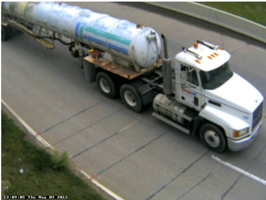
Photo 36B: Class 9, 5 axle, Semi-Tractor with Trailer; Tanker; Liquid.
