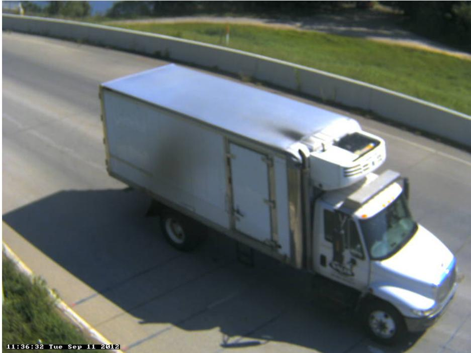
Photo 5A: Class 5, 2 axles, Single Unit; Box; Reefer.
