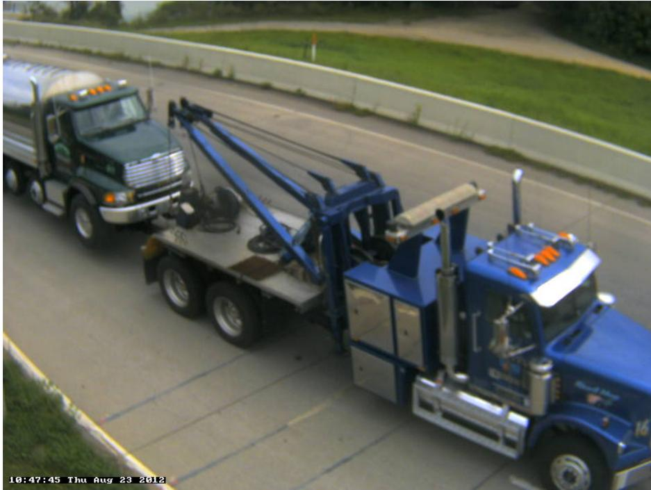
Photo 28A: Class 9, 5 axles, Semi-Tractor with Trailer; Service Truck; Tow Truck.
