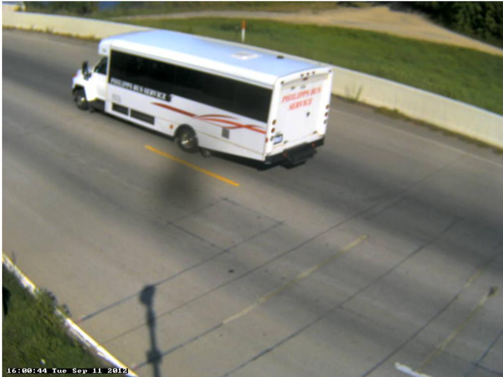
Photo 6B: Class 5, 2 axles, Single Unit; Bus.
