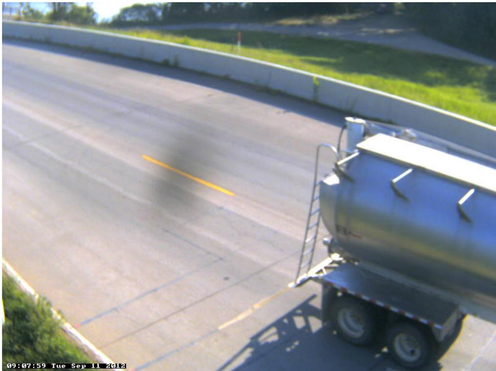
Photo 21: Class 9, 5 axle, Semi-Tractor with Trailer; Grain with Feed Auger, Grain.
