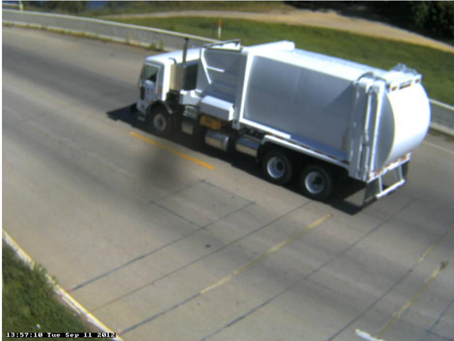
Photo 15A: Class 6, 3 axle, Single Unit; Waste; Garbage Truck.
