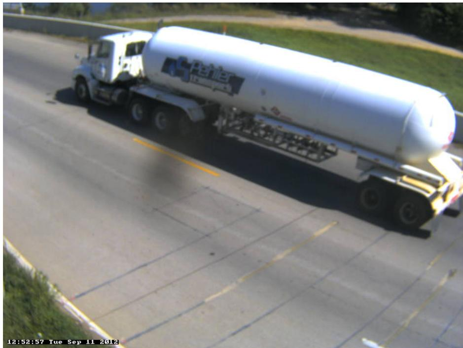
Photo 35B: Class 9, 5 axle, Semi-Tractor with Trailer; Tanker; Fuel; Propane or LNG.
