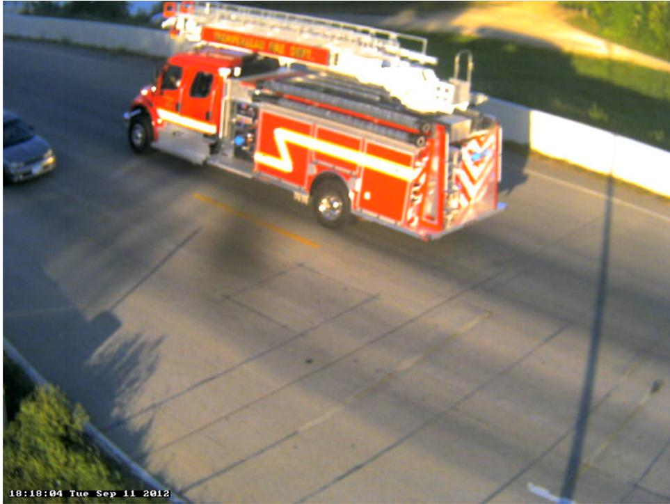
Photo 27A: Class 5, 2 axles, Single Unit; Service Truck; Emergency Vehicle.
