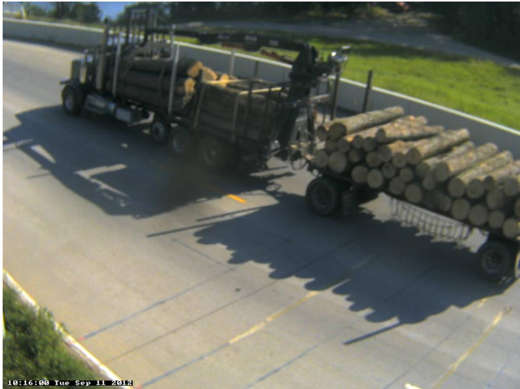
Photo 31A: Class 12, 6 axle Twin Trailer; Stake; Timber. This one weighed 102,000 pounds!
