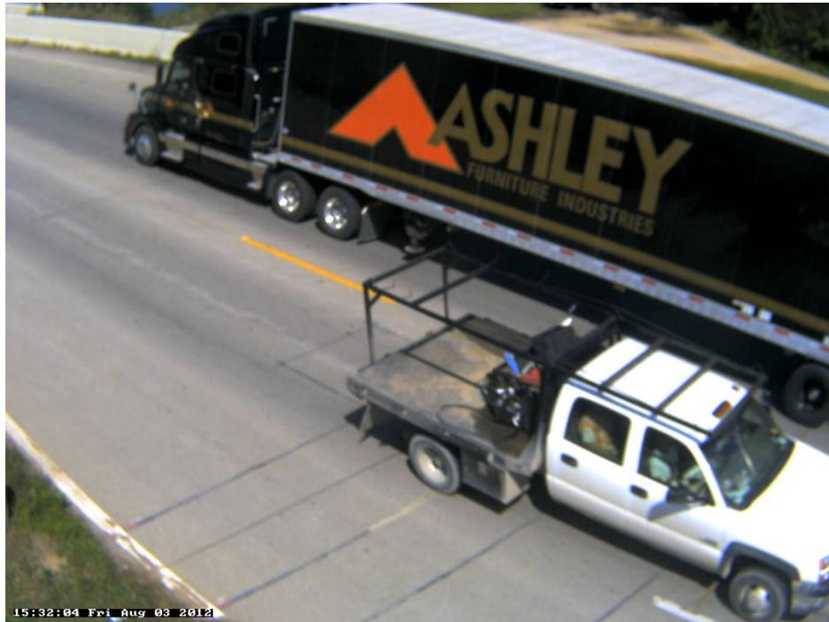
Photo 30A: Class 5, 2 axles, Single Unit; Service Truck; Utility.
