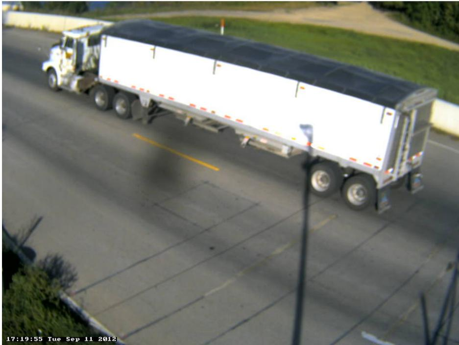
Photo 19B: Class 9, 5 axle, Semi-Tractor with Trailer; Grain Box; Grain.
