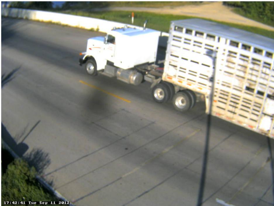
Photo 23B: Class 9, 5 axle, Semi-Tractor with Trailer; Agriculture; Livestock Trailer.
