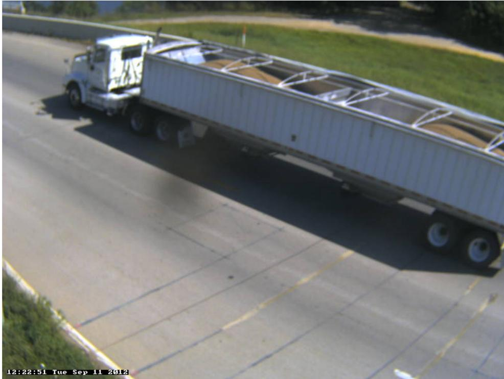
Photo 16A: Class 9, 5 axle, Semi-Tractor with Trailer; Grain Box; Aggregate.
