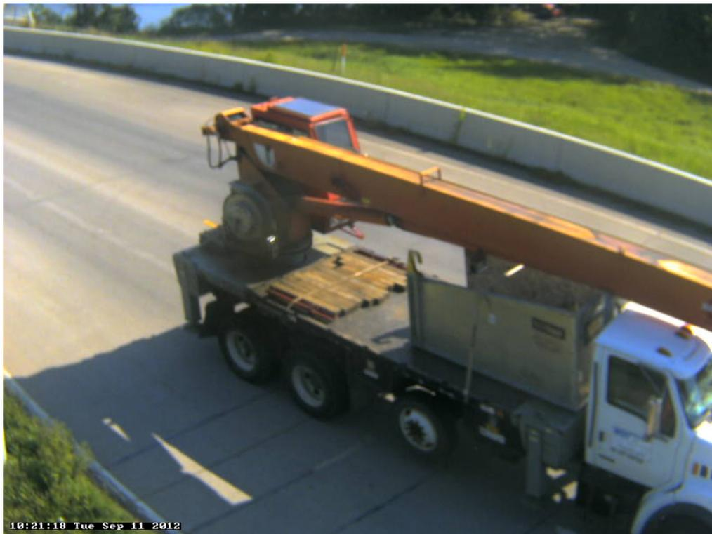
Photo 14B: Class 6, 3 axles, Single Unit; Flatbed; w/Hoist.
