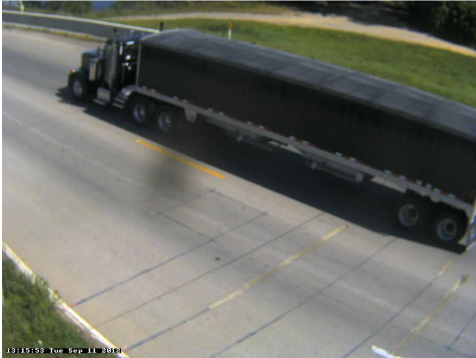
Photo 19A: Class 9, 5 axle, Semi-Tractor with Trailer; Grain Box; Grain.
