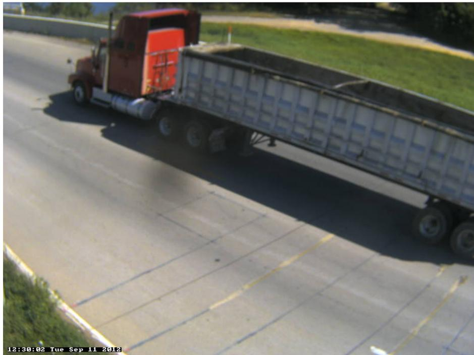
Photo 17B: Class 9, 5 axle, Semi-Tractor with Trailer; Grain Box; Aggregate.
