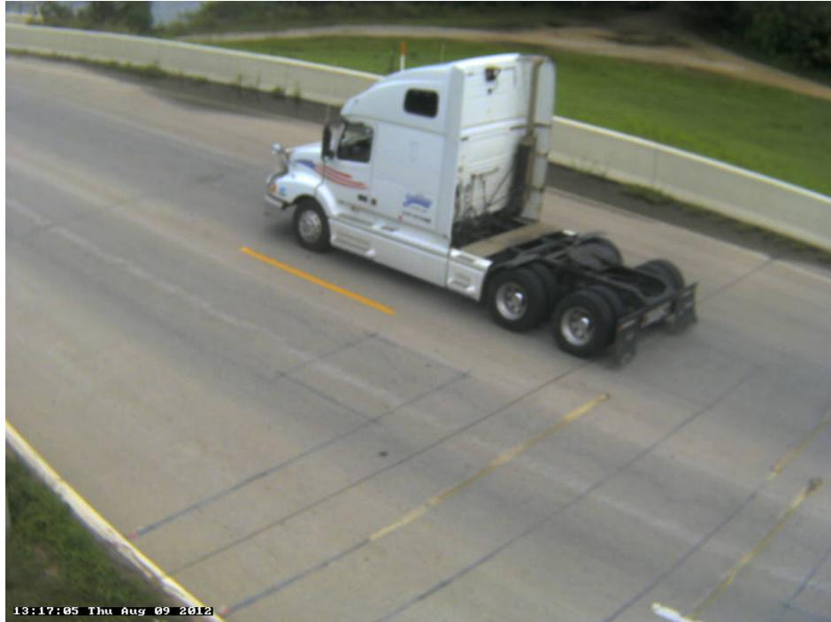
Photo 26A: Class 6, 3 axle, Single Unit; Semi-Tractor w/o Trailer.
