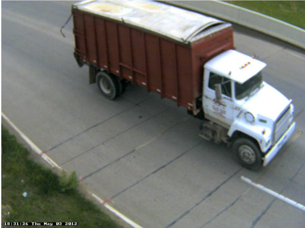
Photo 22A: Class 5, 2 axles, Single Unit, Grain Box, Agriculture; Grain.
