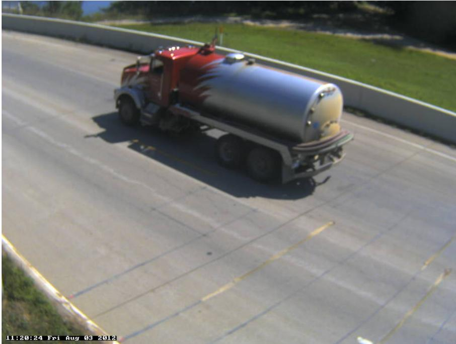
Photo 36A: Class 6, 3 axle, Single Unit; Tanker; Waste; Vacuum Truck; Septic or Liquid Waste.
