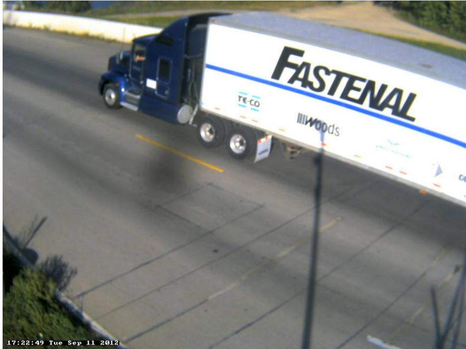
Photo 4A: Class 9, 5 axle, Semi-Tractor with Trailer; Box.
