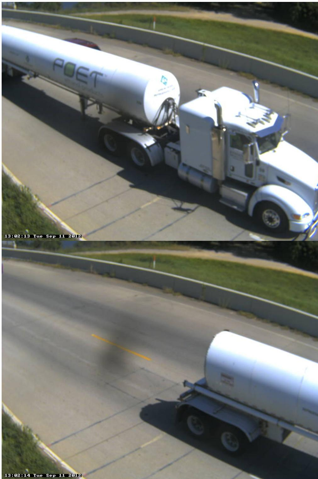
Photo 32: Class 9, 5 axle, Semi-Tractor with Trailer; Tanker; Non-Flammable Compressed gas.
