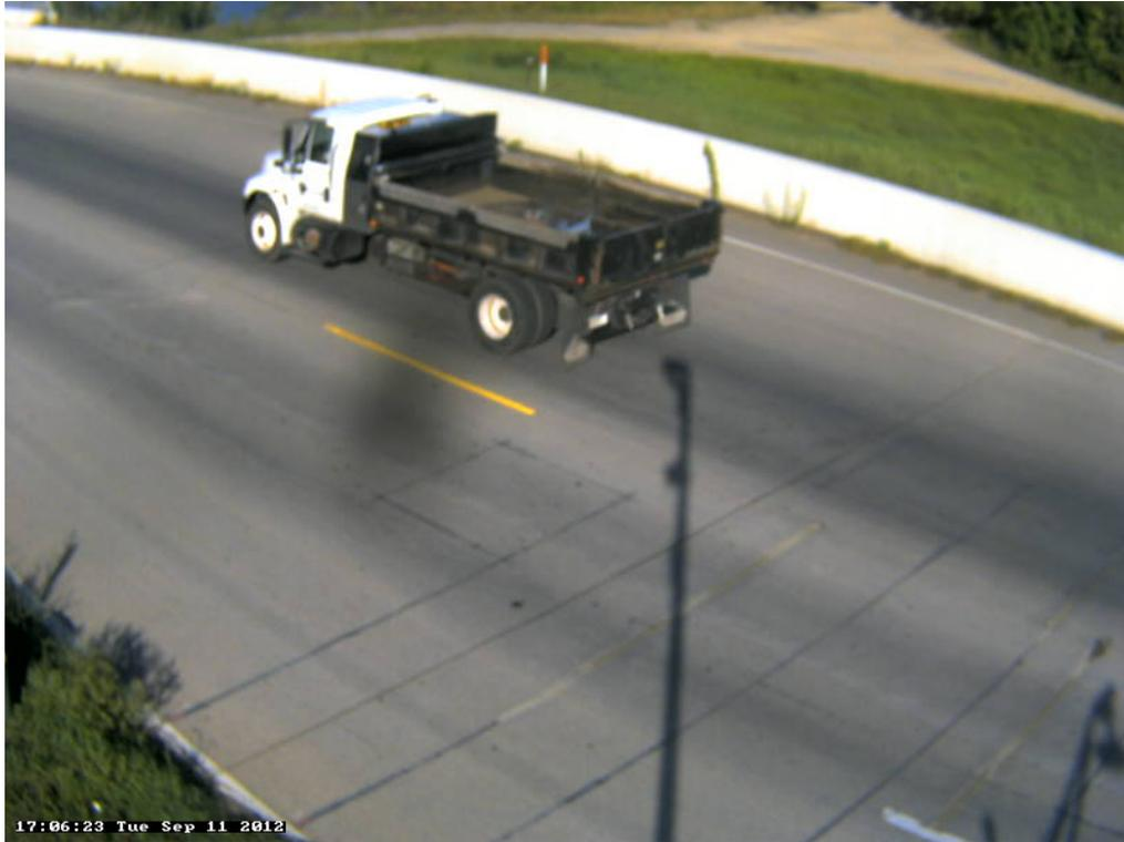
Photo 9A: Class 5, 2 axles, Single Unit; Dump Truck, Low Box.
