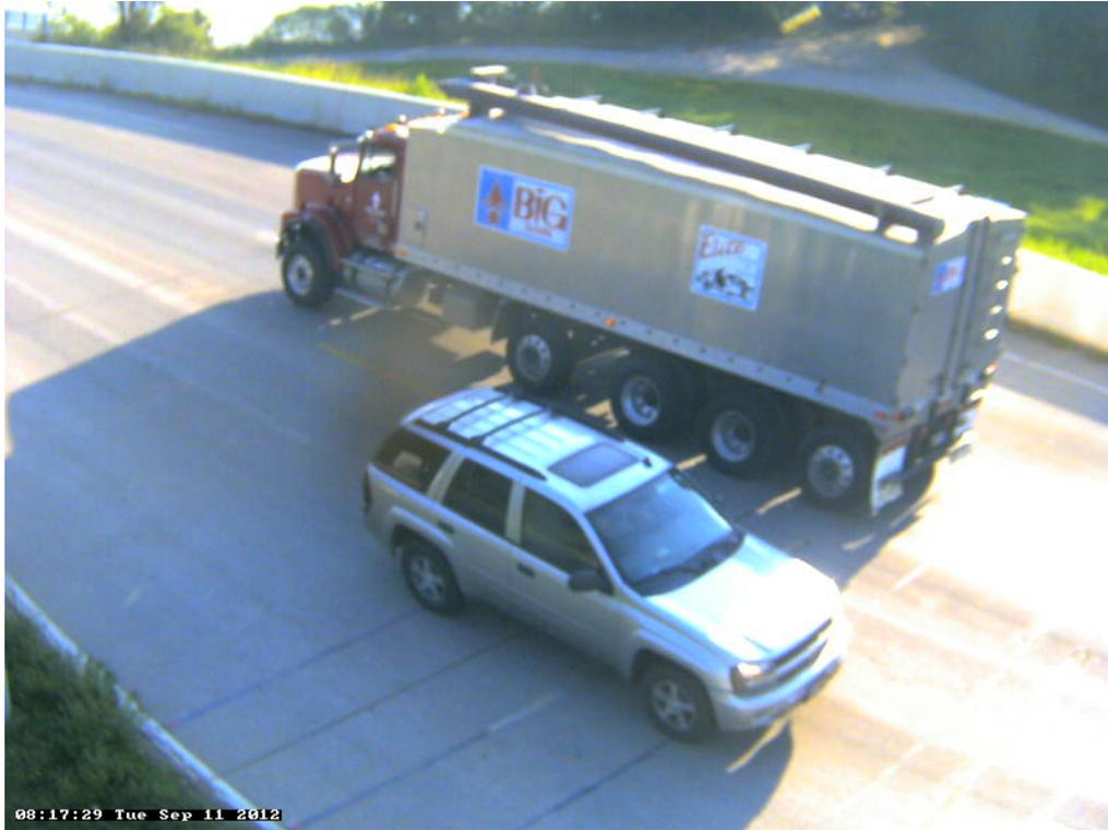
Photo 20A: Class 7, 4+ axles, Single Unit, Grain with Feed Auger; Grain.
