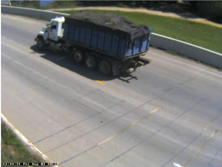
Photo 10A: Class 6, 3 axle, Single Unit; Dumpster Hauler; Full.
