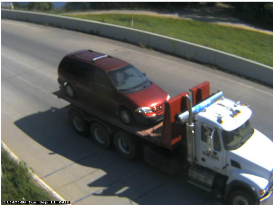
Photo 12B: Class 6, 3 axles, Single Unit; Flatbed, Full. Notice this is the same vehicle as above just loaded and going in the opposite direction.
