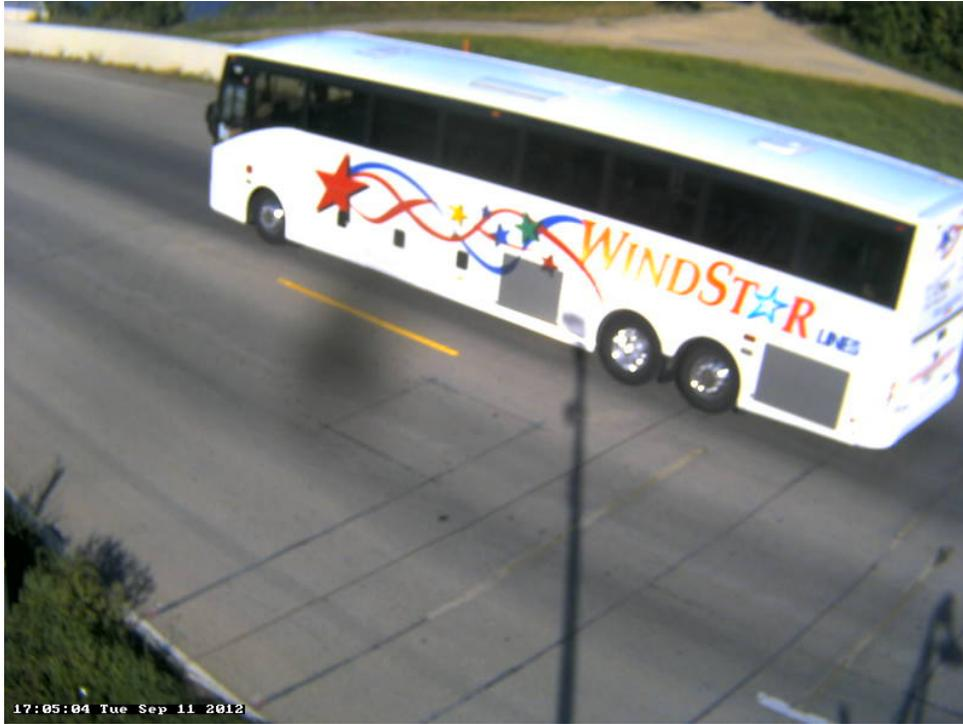
Photo 7A: Class 4, 3 axles, Single Unit; Bus.
