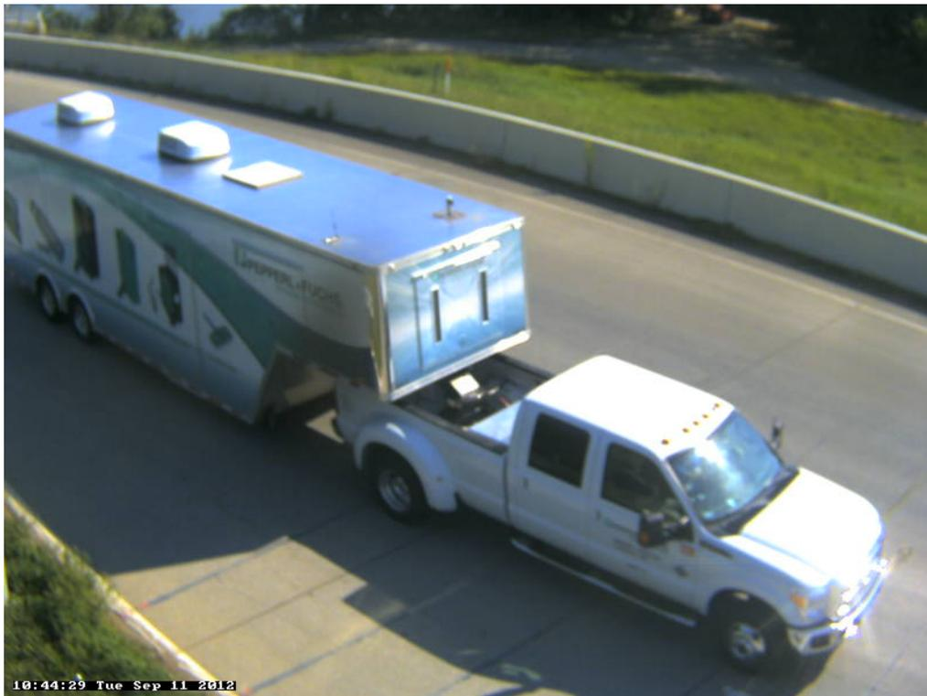
Photo 25B: Class 3, 2 axle, Truck with Trailer; RV.
