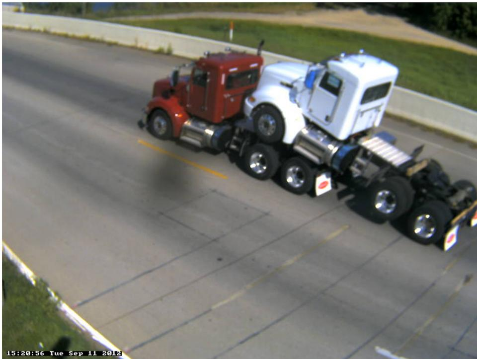
Photo 26B: Class 8, 4 axle, Semi-Tractor; with another piggy-backing.
