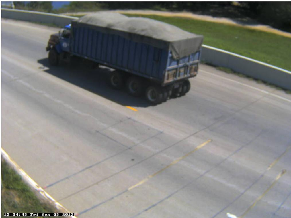
Photo 9B: Class 7, 4+ axle, Single Unit; Dumpster Hauler; Full.
