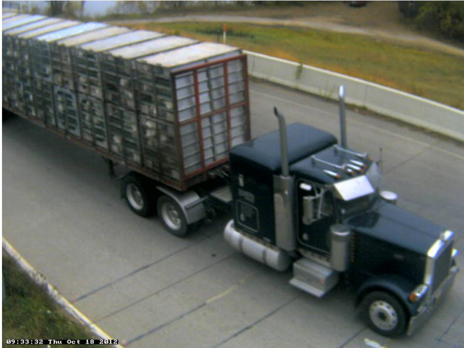
Photo 23A: Class 9, 4 axle, Truck with Trailer; Agriculture; Livestock, Poultry.
