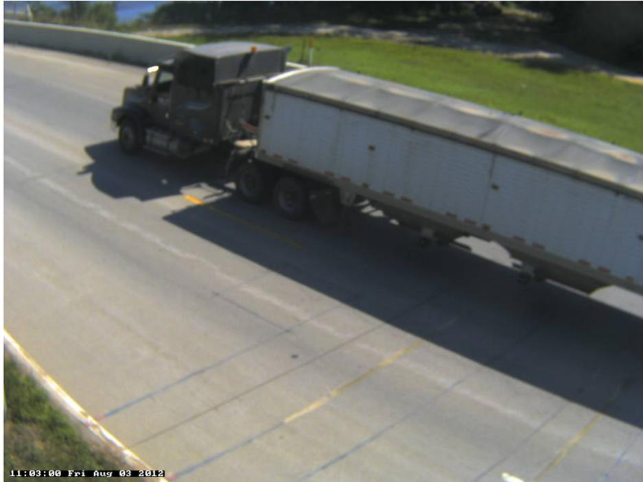
Photo 18A: Class 9, 5 axle, Semi-Tractor with Trailer; Grain Box; Grain.
