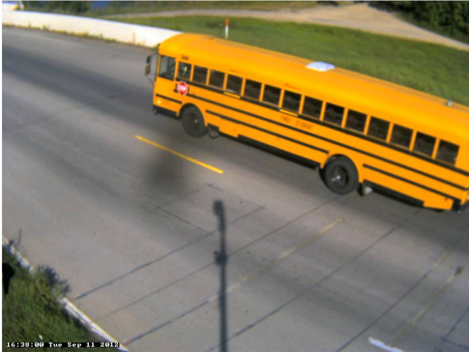
Photo 6A: Class 5, 2 axles, Single Unit; Bus.
