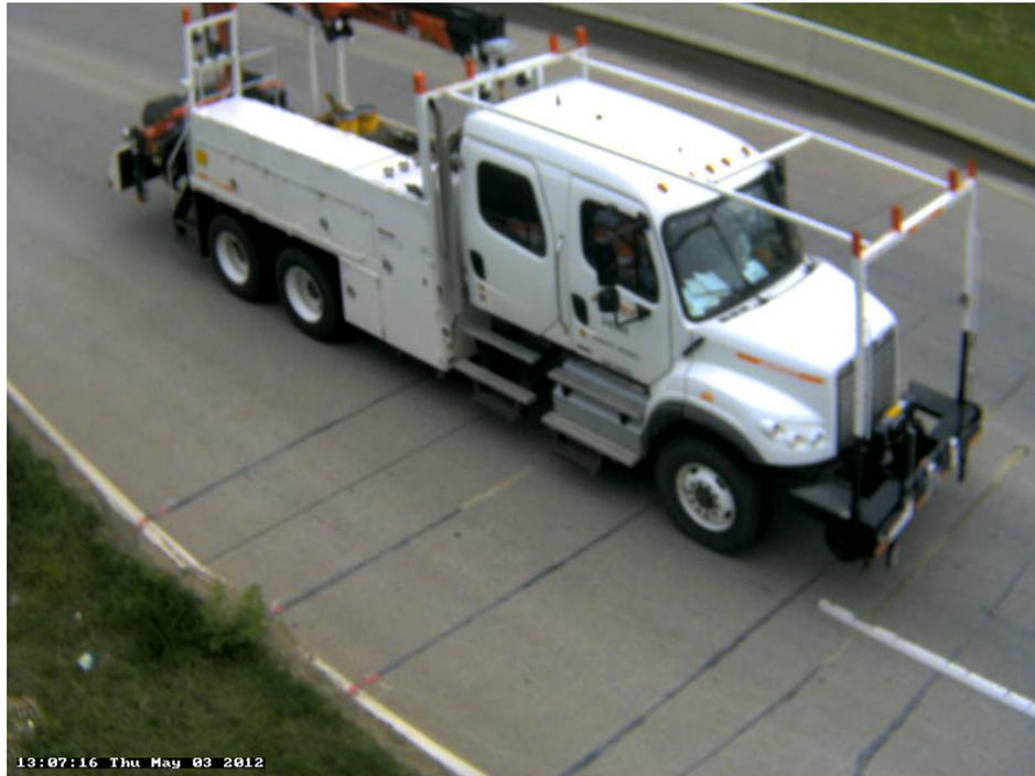
Photo 27B: Class 6, 3 axles, Single Unit; Service Truck; Shipping, Railroad Maintenance Vehicle.
