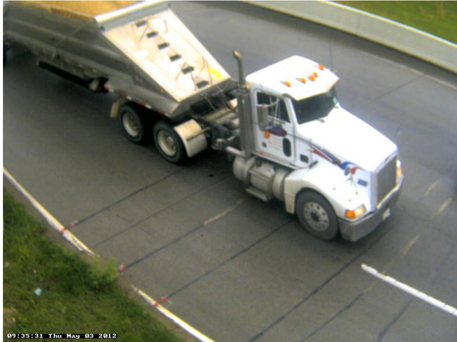
Photo 17A: Class 9, 5 axle, Semi-Tractor with Trailer; Heavy-Duty Bottom-Dump; Aggregate.
