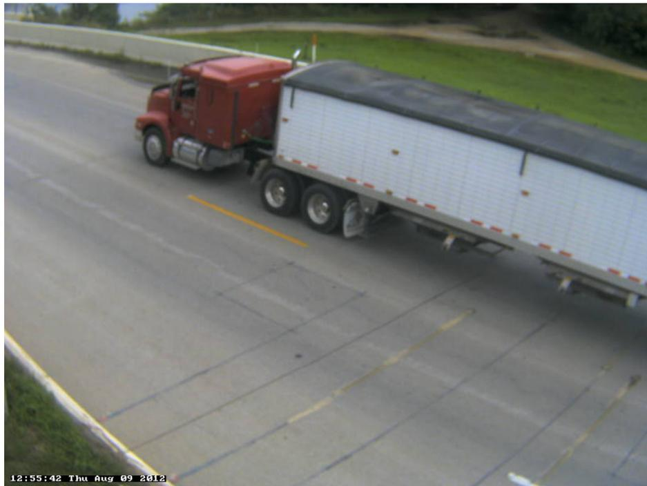
Photo 18B: Class 9, Semi-Tractor with Trailer; Grain Box; Grain.
