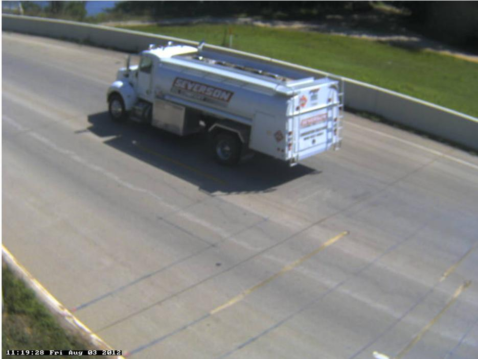
Photo 34A: Class 5, 2 axle, 6 tires, Single Unit; Tanker; Fuel; Petroleum.
