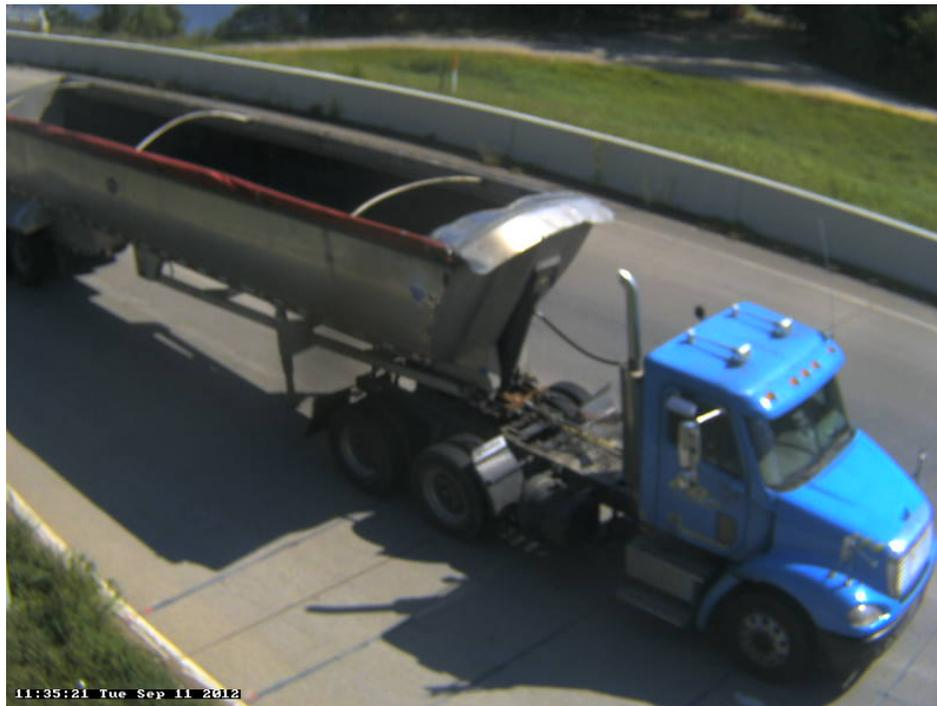
Photo 16B: Class 9, 5 axle, Semi-Tractor with Trailer; End-Dump Hopper, Aggregate.
