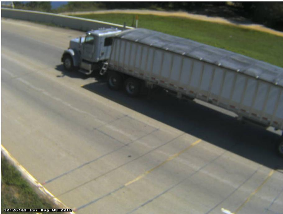
Photo 15B: Class 9, Semi-Tractor with Trailer; Grain Box, Aggregate.
