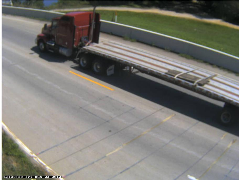
Photo 13A: Class 9, Semi-Tractor with Trailer; Flatbed; empty.
