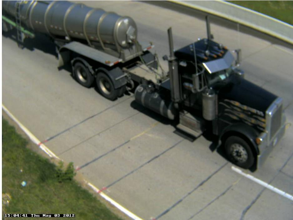
Photo 37A: Class 9, 5 axle, Semi-Tractor with Trailer; Tanker; Liquid.
