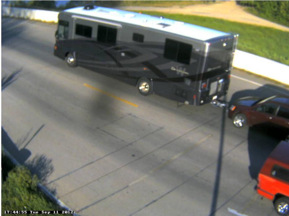
Photo 25A: Class 4, 2 axles, Single Unit; Recreational Vehicle; w/Car being towed.
