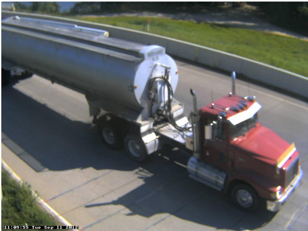
Photo 20B: Class 9, 5 axle, Semi-Tractor with Trailer; Grain with Feed Auger, Grain.
