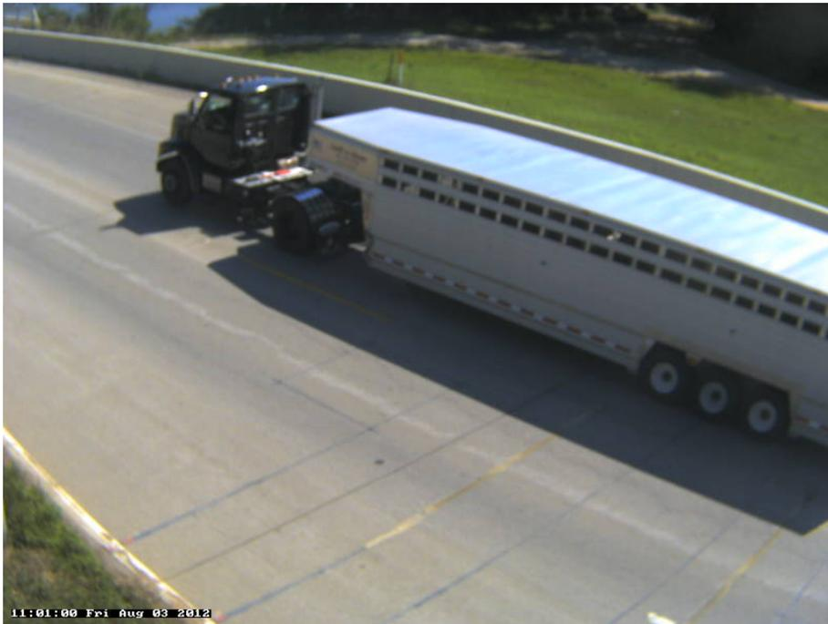
Photo 22B: Class 9: 5 axle, Semi-Tractor with Trailer; Agriculture; Livestock.
