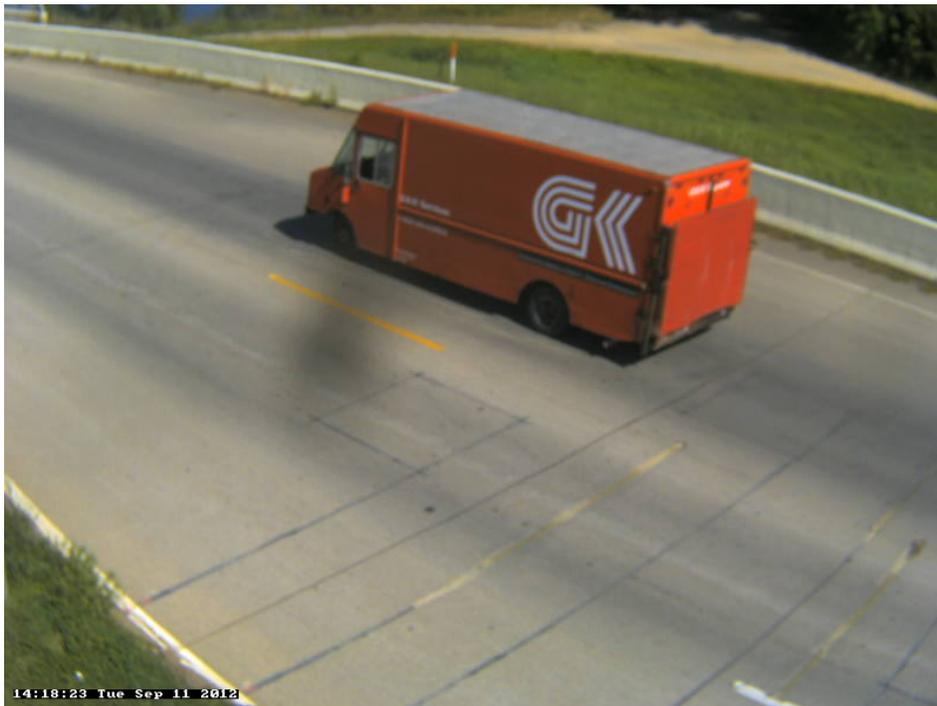
Photo 29B: Class 5, 2 axles, Single Unit; Service Truck; Service Industry.
