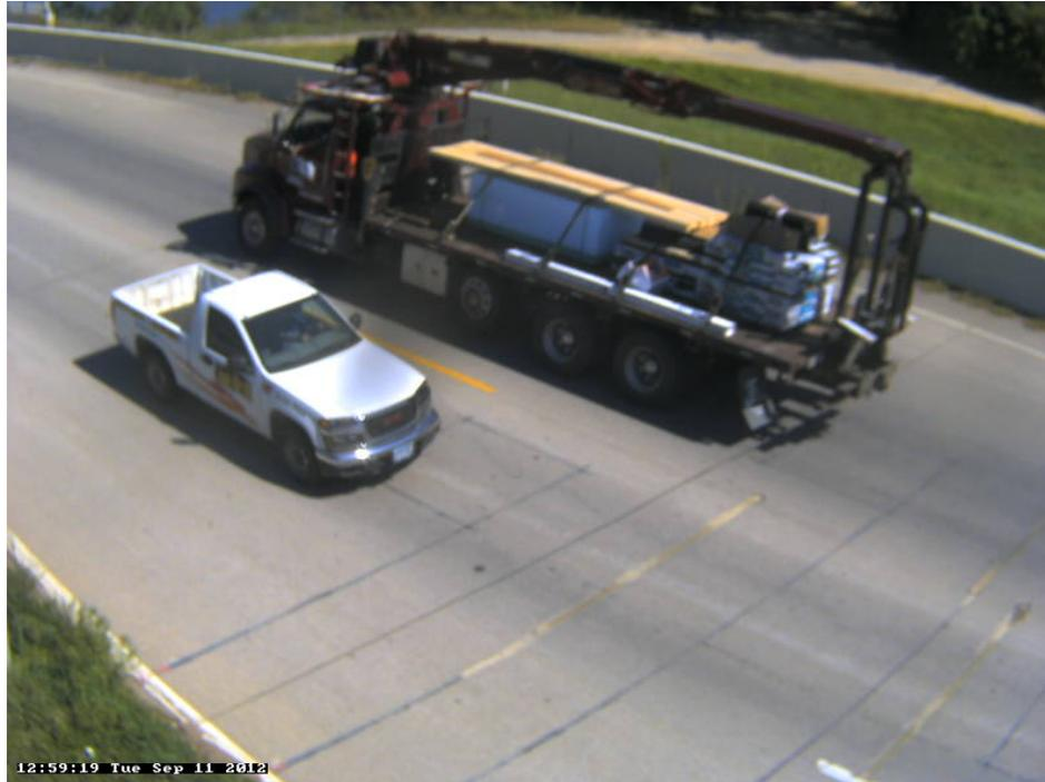
Photo 14A: Class 6, 3 axles, Single Unit; Flatbed; Construction – Materials; w/Hoist, Loaded.
