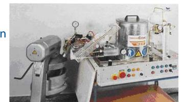
**Introducing moisture into a stream of hot asphalt creates a foam that mixes well with aggregates.**
