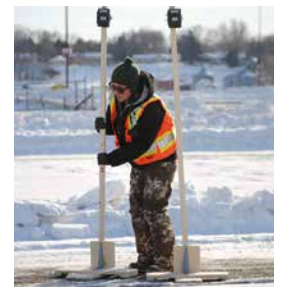
Pole-mounted time-lapse cameras with detachable bases documented deicer and plow testing on side-by-side test tracks.
