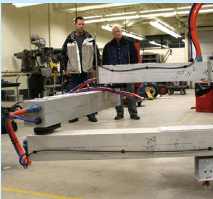
MnDOT District 3 launched research that has created a robotic spray-painter to draw turn arrows, crosswalk stripes and other designs on roadways. The robot can be mounted on the front of a maintenance vehicle and controlled via laptop computer. The project's goal is to save manpower and keep crews safer. Read more about this project and watch a video demonstration in our Crossroads blog at [mntransportationresearch.org](http://mntransportationresearch.org).
