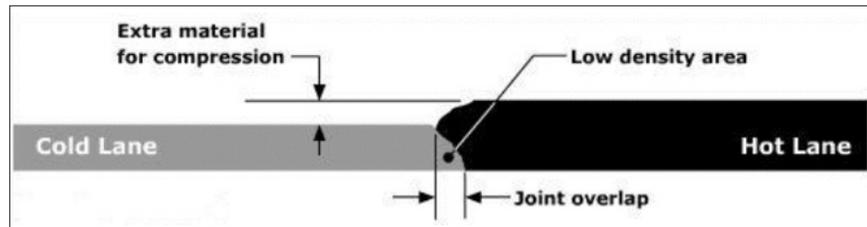
This cross section of a latitudinal joint shows where the pavements overlap, typically the location of lowest density on a finished road.
