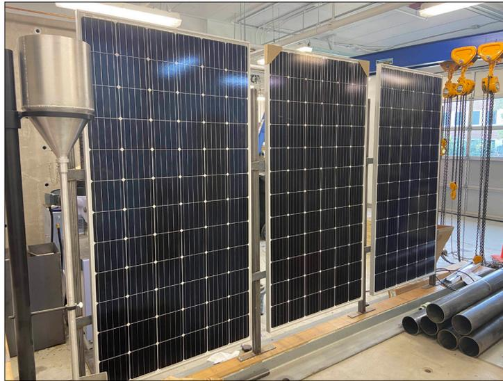
The research team developed and constructed this prototype of a PV noise barrier system using 8-by-4-foot solar panels.
