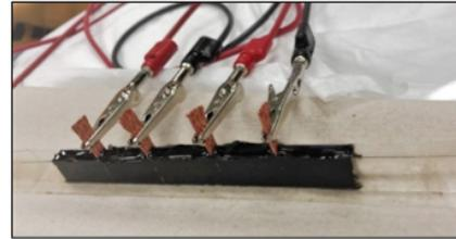
Researchers tested the electrical conductivity of asphalt mixtures using strip samples with GNP/taconite added. Four electrical probes were inserted into samples: Two outer probes delivered current while two inner probes measured voltage within the sample.
