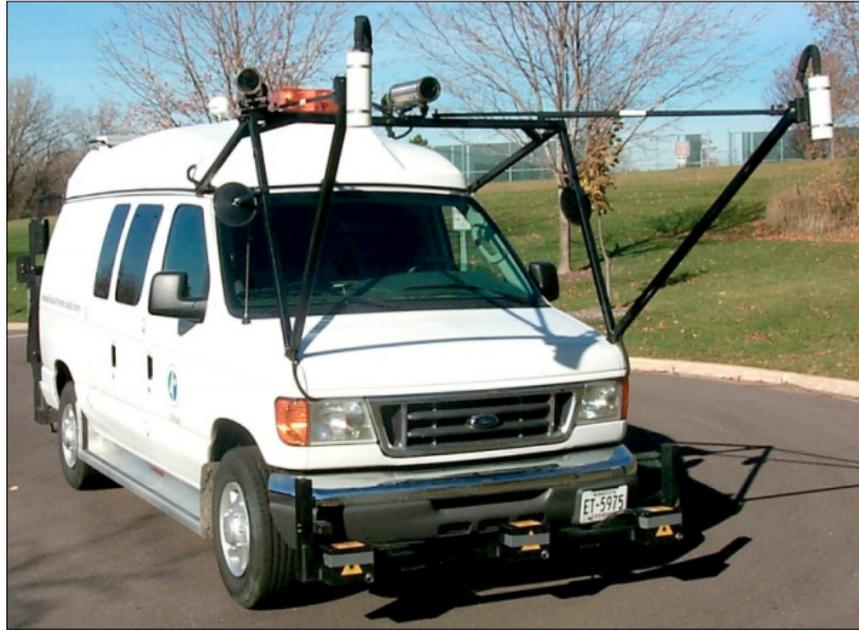
Pavement roughness is measured with a digital pavement inspection vehicle, which is equipped with accelerometers that record differences in pavement incline. Other methods of determining pavement condition involve visual evaluation of the surface, such as signs of cracking, rutting and faulting.
