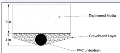
This drawing shows the design of one set of test filtration sites. Filtration samples were obtained from the underdrain pipes.
