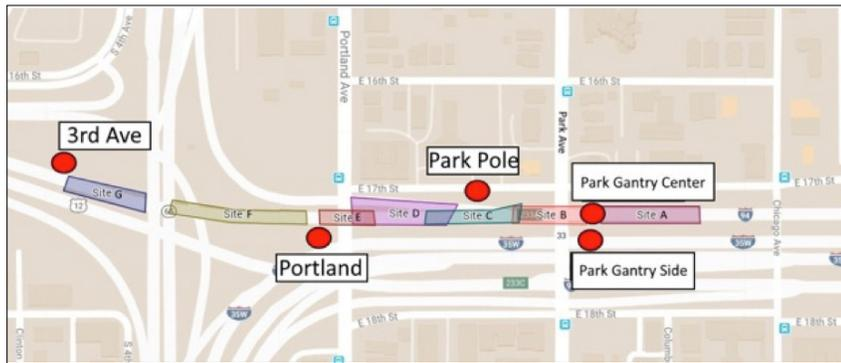
The new traffic state estimator was evaluated on a section of I-94 in Minneapolis. This map shows the location of radar sensors (red circles) and the area monitored by each device (overlapping colored rectangles).
