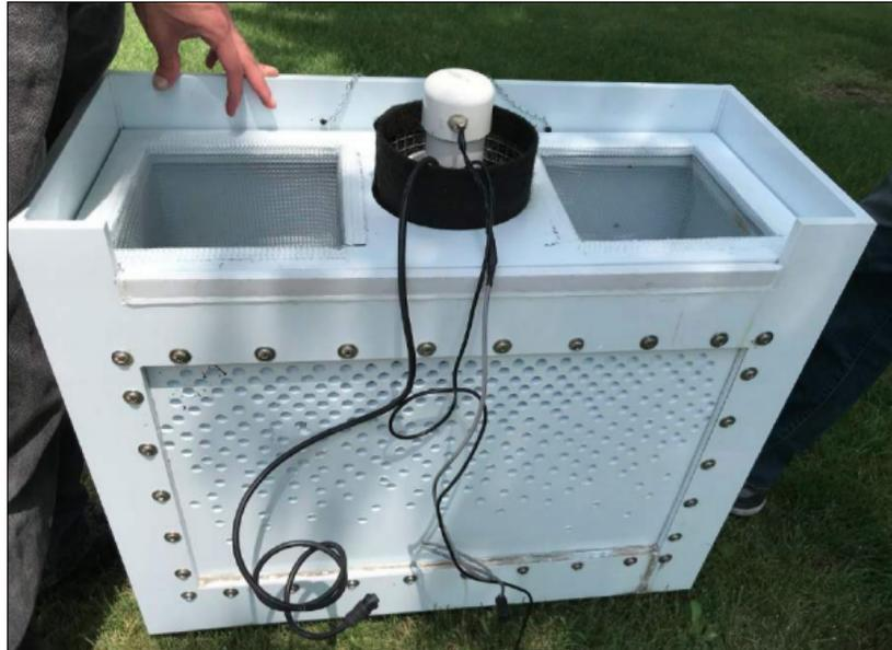
This sampler box, mounted below the grate of a storm catchment drain, collected water flow, temperature and conductance data over two winters.
