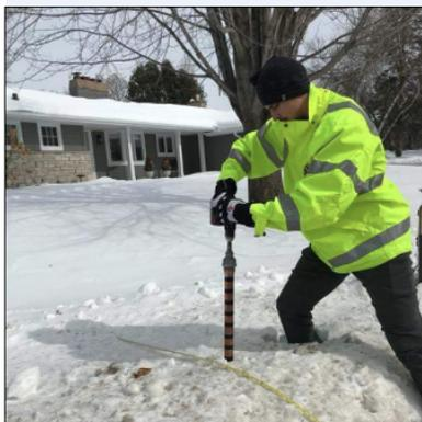
Core samples from snow and ice piles were analyzed for chloride levels.
