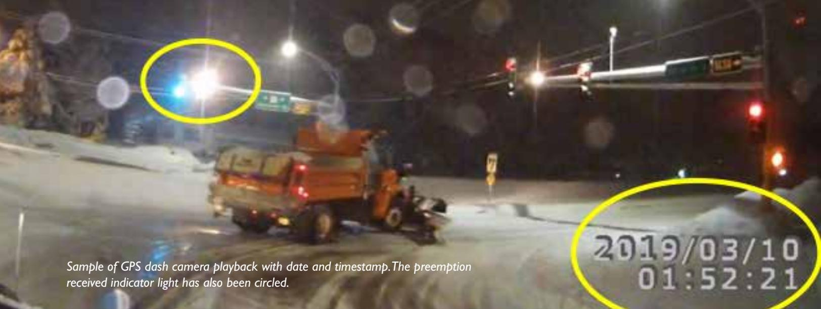
Sample of GPS dash camera playback with date and timestamp. The preemption received indicator light has also been circled.
