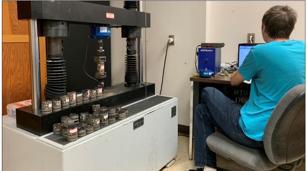
Investigators at Michigan Technological University developed new bond tests to determine the impact of freeze-thaw activity, temperature and moisture on pavement samples.
