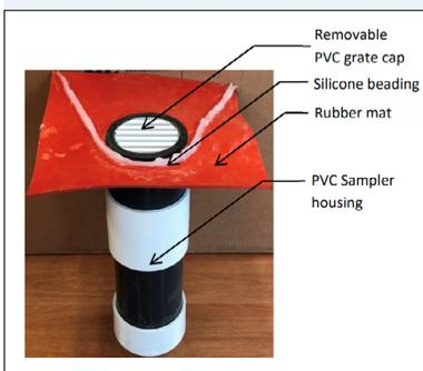
The runoff sampler used to collect stormwater runoff samples at the low-volume road sites.
