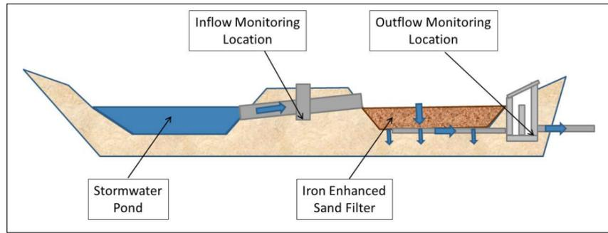
The TH 610 two-cell IESF system consists of a stormwater pretreatment cell (left) that drains through the berm via a connecting pipe to the IESF basin (right).
