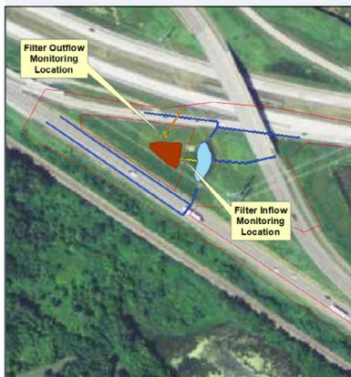
An overhead view shows the location of the TH 610 IESF wet pretreatment cell (blue) and filtration basin.
