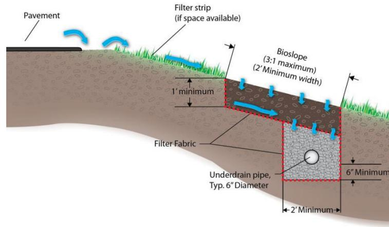
This cross section of a common engineered bioslope shows the position of a vegetation filter strip, a section of biofiltration material and an underdrain pipe beneath it. The blue arrows indicate the flow of water.
