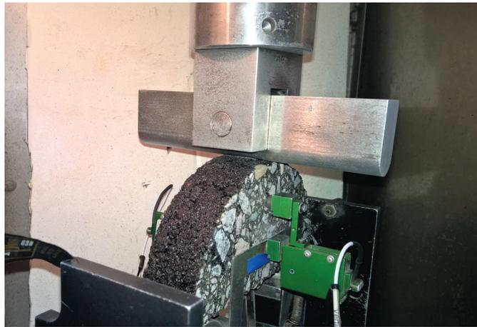
The SCB test applies pressure diametrically on an asphalt pavement puck along the axis of a 6-inch pavement cylinder to measure susceptibility to cracking at low temperatures.
