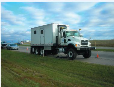
Cone penetration testing can be conducted safely from inside a truck container alongside a highway.
