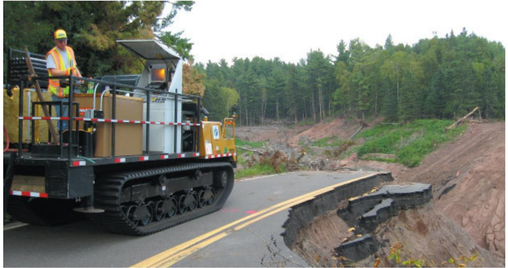
One operator can investigate soil and foundation conditions with a sophisticated CPT vehicle, even at a highway washout.
