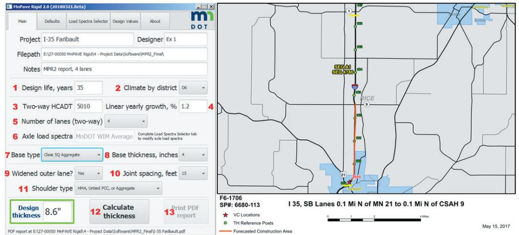
MnDOT engineers use sophisticated and complex M–E pavement design methods from MnPAVE-Rigid 2.0 software to design durable, high-performing concrete pavements.
