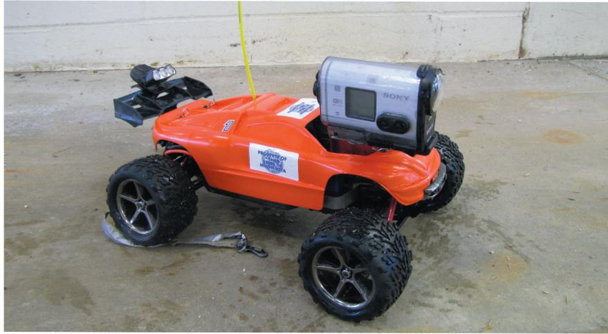
MnDOT inspectors constructed this HIVE inspection robot from off-the-shelf electronics, developing an inexpensive and effective imaging tool for culvert inspection.
