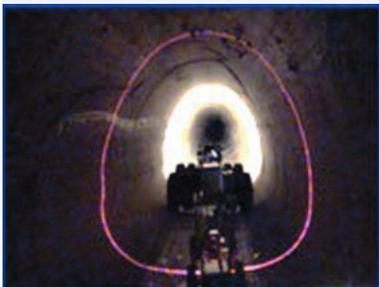
Laser ring profilers offer precise readings of how much culverts have reshaped under environmental conditions.
