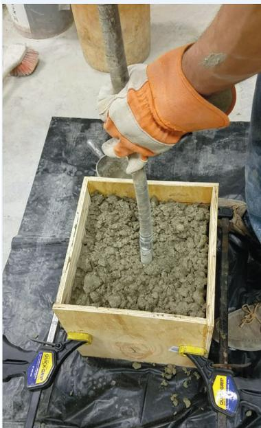
Investigators vibrated RCA mixes in sample boxes to prepare the mixes for mechanical analysis.
