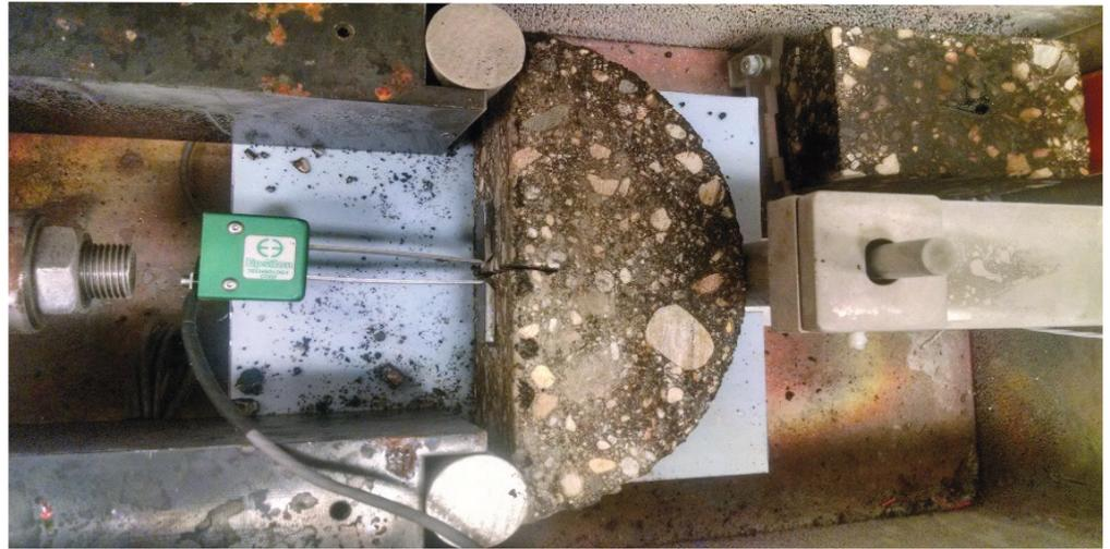
The SCB test evaluates the propagation of cracks in a notched semicircular sample as it is subjected to loads.
