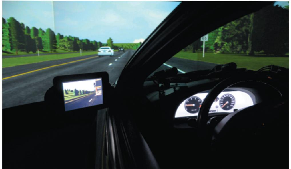
The HumanFIRST driving simulator provides a realistic driving experience while collecting detailed data about the user’s driving behavior and performance. In this test the IVS was mounted on the center console to provide or supplement speed limit information.
