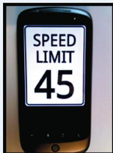
An IVS system displays roadside sign information on a smartphone or similar device in a vehicle.
