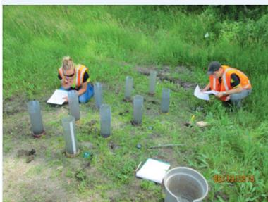
Measurements were taken via tube infiltrometers at Minnesota Highway 51 to validate the model developed in this study.
