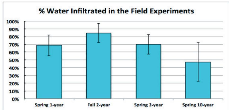
Average percentage of stormwater infiltrated in the field experiments. Two sites were tested for each of four highways. Three rainfall intensities were applied: 1-, 2- and 10-year storms. The error bars represent the standard deviations.
