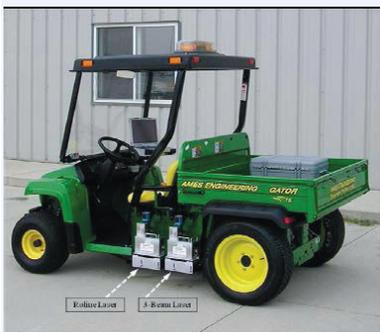
The Lightweight Inertial Surface Analyzer's lasers measure roughness, which indicates deterioration if it increases over time.
