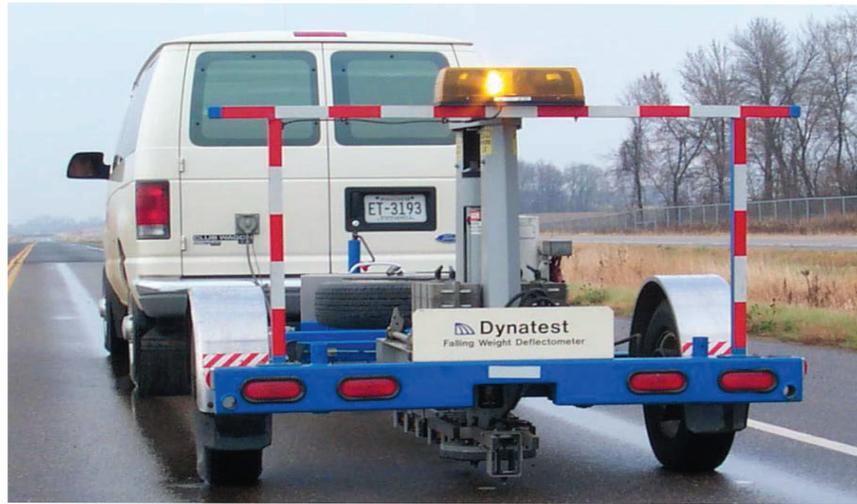
The FWD test consists of a loading plate, weight package, sensors and data acquisition equipment. Researchers drop the weight and measure deflection in each pavement layer to identify stresses likely to trigger eventual pavement failure.
