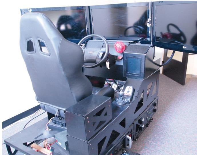
The HumanFIRST portable driving simulator includes three 32-inch high-definition displays, rearview mirror displays and vehicle controls. Vibrating motors installed in the left and right sides of the seat pan provide lane departure warnings. Drivers performed a secondary, distracting task via an 8-inch touch screen LCD on the right side, 25 degrees below the driver’s horizontal line of sight.
