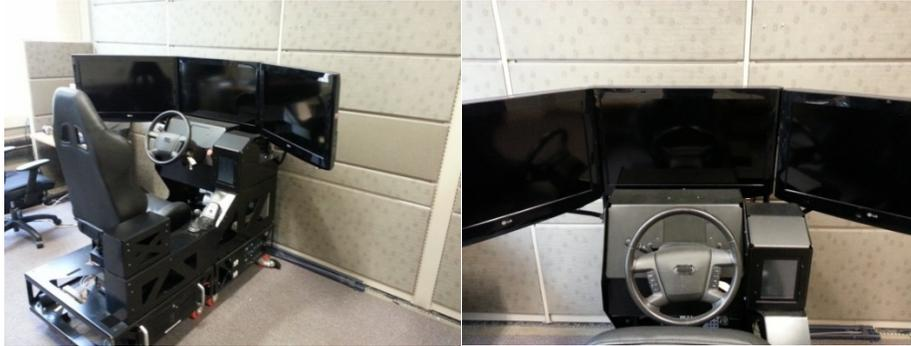
**Figure 2.1. HumanFIRST portable driving environment simulator**
