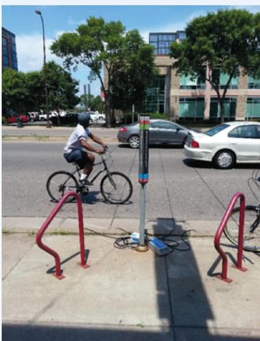
Pneumatic tubes are one tool suitable for short-term bicycle counts.
