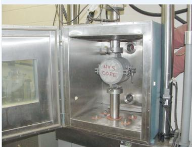
The Florida Bond Test measures the force needed to shear an asphalt sample perpendicular to the roadway surface.
