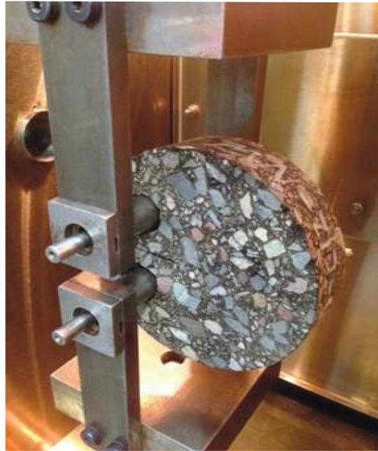
The DCT testing apparatus, which measures the fracture energy of a sample asphalt core in the lab, was found to be a good indicator of field performance.
