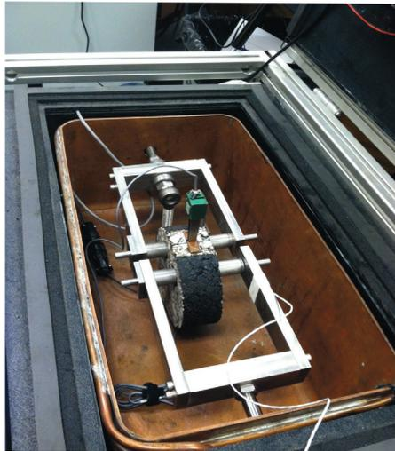
The DCT test notches and pulls apart an asphalt sample to determine its fracture energy. The test is conducted at 10 degrees Celsius above the asphalt binder’s performance-graded low-temperature grade for 98 percent reliability, which ranged from -18 degrees Celsius to -30 degrees Celsius for the pavements analyzed in this project.
