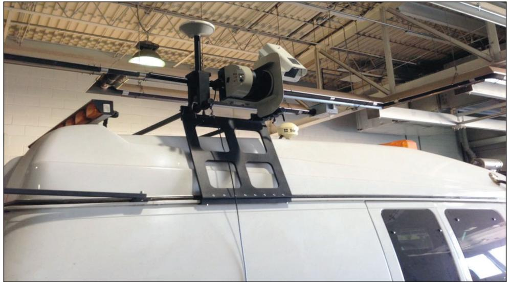
The system tested in this project is installed with the camera facing downward so that its field of view contains the pavement adjacent to the vehicle to about 3 m away from the side of the vehicle.
