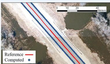
In many locations, fog lines were accurately computed to within 2 cm—so small that actual fog lines (marked in red) are not visible under computed lines (blue).
