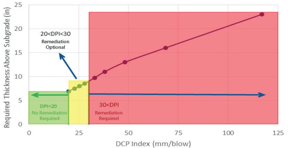
The specification being developed by MnDOT as a result of this project establishes the required subgrade stiffness (as measured by the dynamic cone penetrometer) to be obtained by cement stabilization and compaction.
