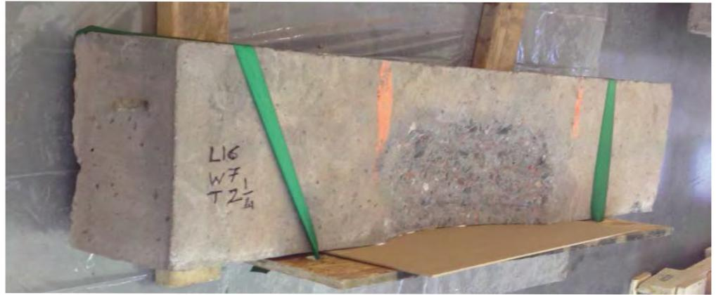
Researchers tested the bond strength of half-slab concrete specimens by loading them at their midpoint to see if the resulting flexure caused a partial-depth repair patch to pop out.
