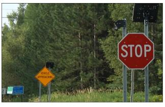
In Phase 1, flashing LEDs on traffic signs (left) were part of the ALERT system. In Phase 2, LEDs were added to stop signs on the minor approach (right) to attract driver attention and reduce roll-throughs.
