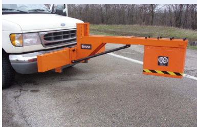
GPR can be used on vans traveling at highway speeds.
