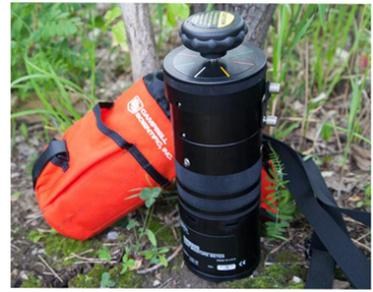
To use the DOT600 (left), a soil sample is placed in the device's compaction chamber and compacted to a selected pressure. The device uses the soil's electrical properties to calculate its moisture content. A ruggedized field device (right) is being developed.
