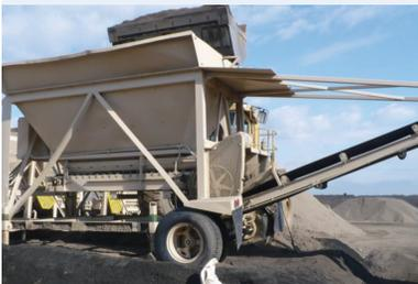
FRAP mixtures were produced using conveyor belts to combine coarse and fine fractions in the right proportions and then send them to a mixing drum.
