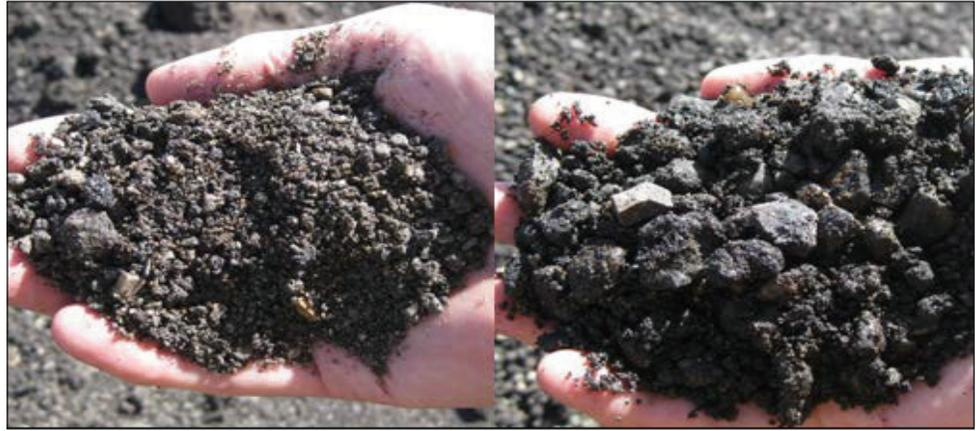
FRAP involves separation based on particle sizes. In this project, RAP was divided into two piles of finer (left) and coarser (right) particles.
