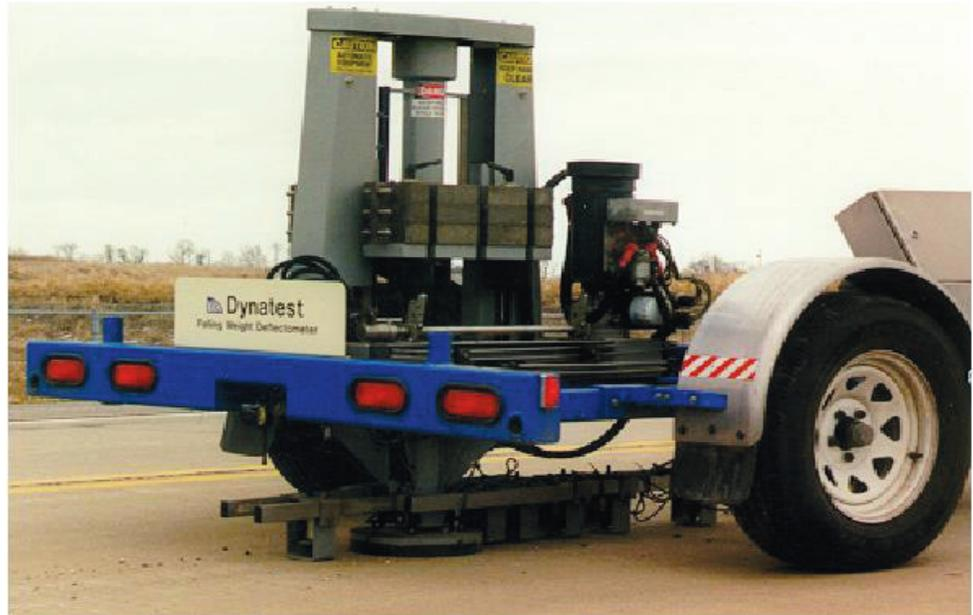
Researchers tested pavement stiffness and response with a falling weight deflectometer. Results showed that stabilized full-depth reclaimed base performs better than unstabilized reclaimed or virgin aggregate bases.
