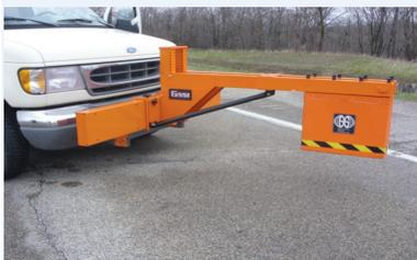
Investigators used ground penetrating radar to develop thickness profiles for the pavement sections evaluated.
