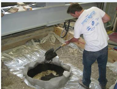
Researchers tested the modulus of recycled pavement material and other materials using a large-scale model experiment.
