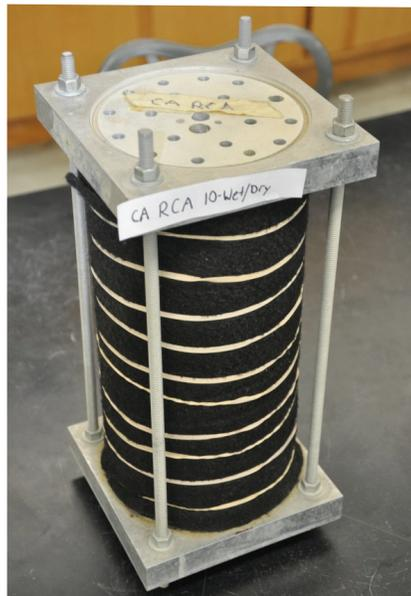
Researchers tested the effects of wet-dry cycles on particle degradation in aggregates with recycled materials by compacting them in a mold and placing them in an apparatus allowing the passage of water.
