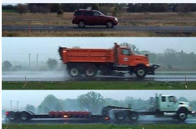
High-resolution video was used to establish length standards for various vehicle classifications.
