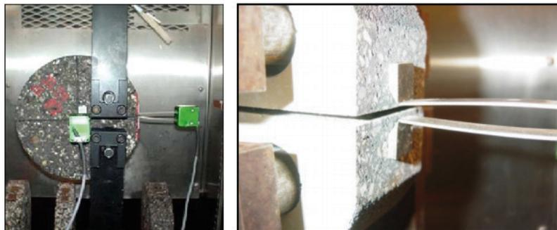
The DCT (left) involves loading cylindrical asphalt specimens that have been cooled and notched with a table saw. A gauge placed at the mouth of the notch (right) is used to measure crack propagation in response to loading.
