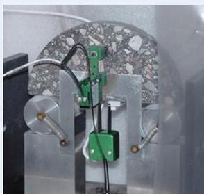
The SCB determines the energy required to cause or propagate cracking in specimens.
