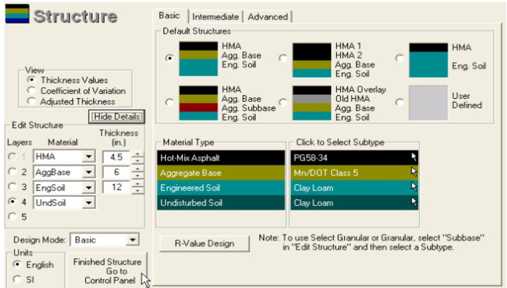
Using software such as MnPAVE (which predicts the service life of a pavement from climate, traffic and structural data) to determine how stabilization improves pavement stiffness is important to mechanistic-empirical design.
