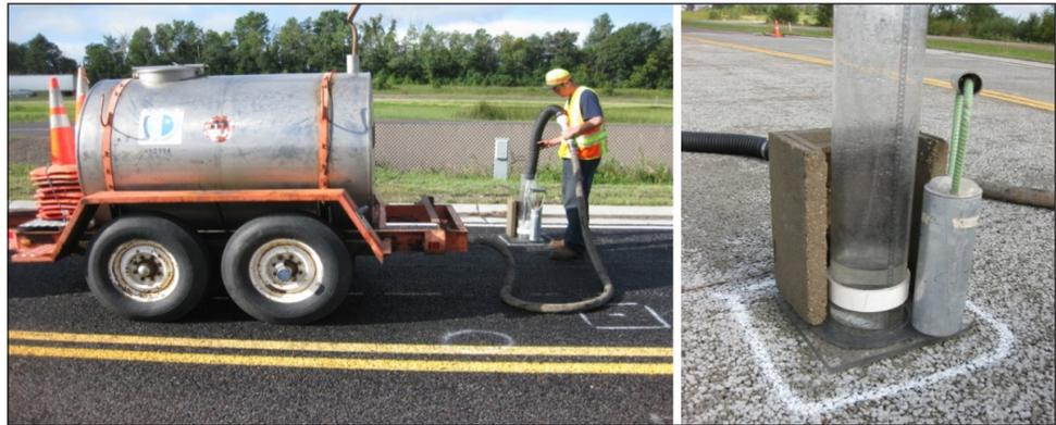
Permeability tests in which water is flushed through the pavement structure were central to the investigation of porous asphalt pavements. The tests confirmed that porous asphalt drains and filters water effectively through the pavement structure.
