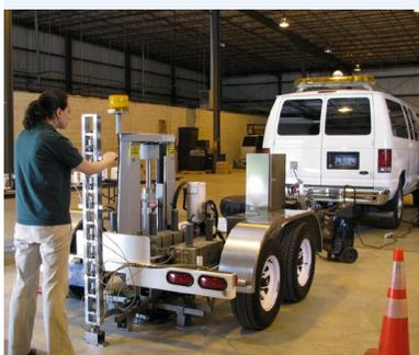
The TONN program processes falling weight deflectometer results, which can be used to evaluate pavement stiffness.
