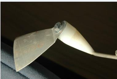
Because flotation devices can be submersed at high velocities, researchers invented a wing that lifts the sampler when water flows across it.
