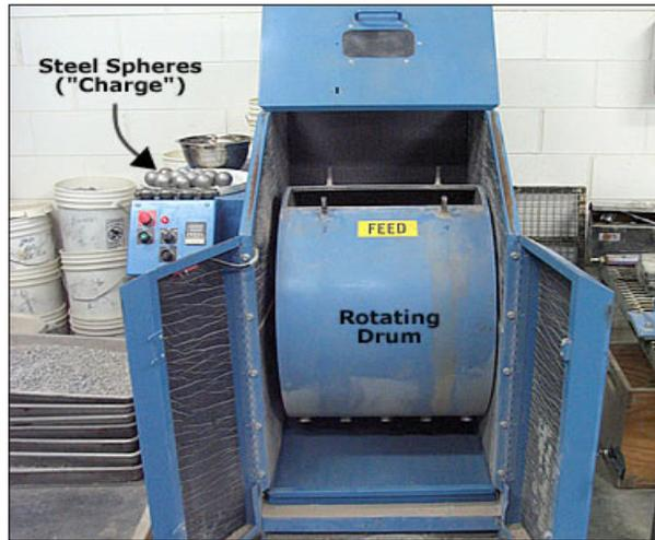
A common test for measuring abrasion resistance is the Los Angeles abrasion test, used to evaluate how well aggregate stones remain intact when subjected to grinding in a rotating steel drum containing steel spheres.
