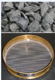
Coarse aggregate rocks are smaller than 3 inches but too large to pass through a sieve with 1/4-inch-diameter holes.
