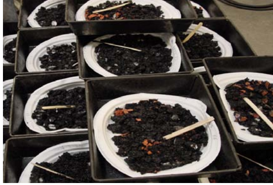
Figure 4. Broken down mixtures used in air voids determination
