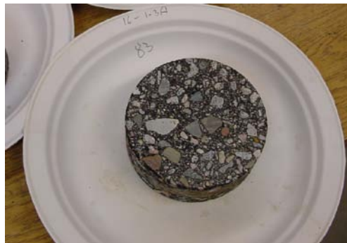
Figure 1. Identifying cores used in air voids determination
